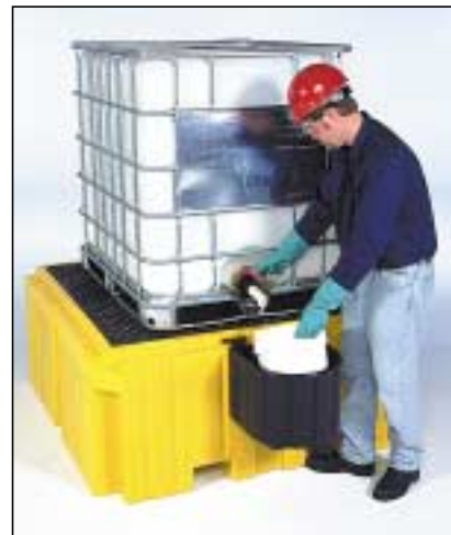
Spills from dispensing that exceed 3 gallons are channeled into the 360-gallon sump through a bulkhead fitting.
